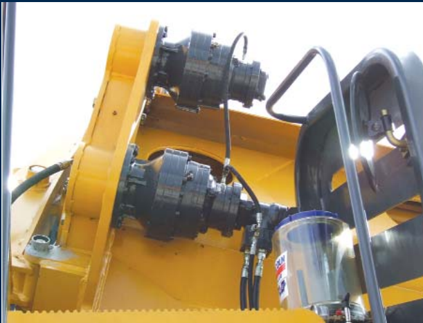
Dual gear boxes with single motor drive double the tooth engagement to reduce gear tooth loading.
